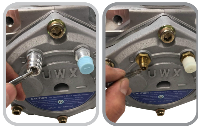
Figure 1. Remove transit gas via discharge service valve or pressure switch port (if fitted). Use a small screw driver or any tool with a pointy end to depress the Schroeder valve.
