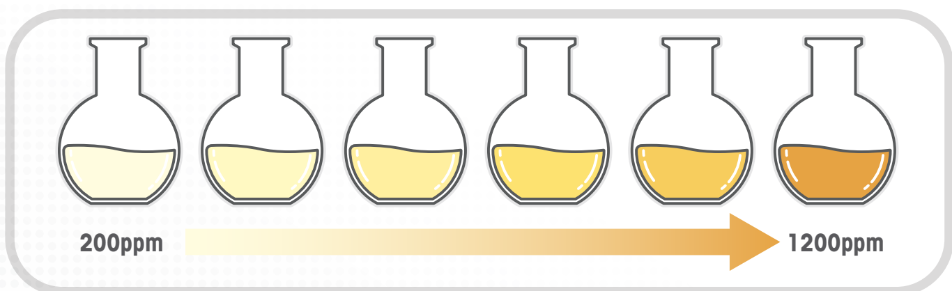
Diagram 20. Colour can be a good indicator of oil quality which darkens as moisture increases.
