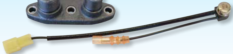
Thermal switch to suit rear manifold (32308-000760) setting cut out 85°C - cut in 65°C 53101-000110
