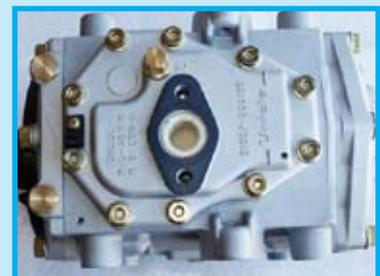
*In the case of older systems where the compressor is replacing a previous failure, the system must be flushed and the filter should be strictly monitored to ensure a blockage does not occur. More than one filter maybe required over several hours to properly clean the particles in the suction line.*
